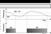
In case of fault in the thermostat probe the start and stop of the compressor are timed through parameters  ${\sf Con}$  and  ${\sf CoF}.$
