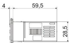
Instrument **XR60CHC** shall be mounted on vertical panel, in a 29x71 mm hole, and fixed using the special bracket supplied. The temperature range allowed for correct operation is 0 to 60°C. Avoid places subject to strong vibrations, corrosive gases, excessive dirt or humidity. The same recommendations apply to probes. Let air circulate by the cooling holes.
