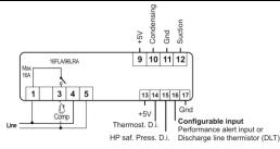
NOTE: terminal 4 and 5 are for power supply at 110VAC or 230VAC depending on the model.
