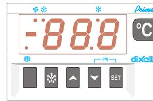
**SET:** To display target set point; in programming mode it selects a parameter or confirm an operation.
