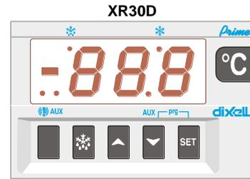
**SET:** To display target set point; in programming mode it selects a parameter or confirm an operation.
