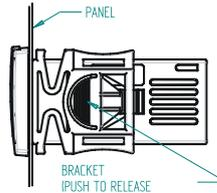
Instrument **XR20CX** shall be mounted on vertical panel, in a 29x71 mm hole, and fixed using the special bracket supplied. The temperature range allowed for correct operation is 0÷60 °C. Avoid places subject to strong vibrations, corrosive gases, excessive dirt or humidity. The same recommendations apply to probes. Let air circulate by the cooling holes.
