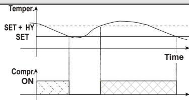
In case of fault in the thermostat probe the start and stop of the compressor are timed through parameters "COn" and "COF".
