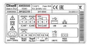
If the parameter is set as disabled, when the instrument is ON and no alarms are present, the relay will close between terminals 5 and 7.
